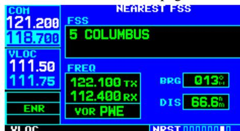
Pressing the small right knob activates the cursor and you can rotate it to select any of up to five nearest FSS locations within 200 nautical miles. The large knob can be used to highlight the frequencies which can be placed in the COM or VLOC windows with ENT button.
